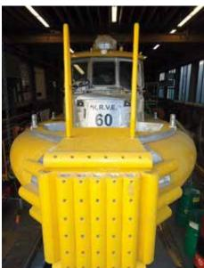
New fendersystem for the fast crew tender KRVE 60 vessel by Poly Marine Fender Systems.
